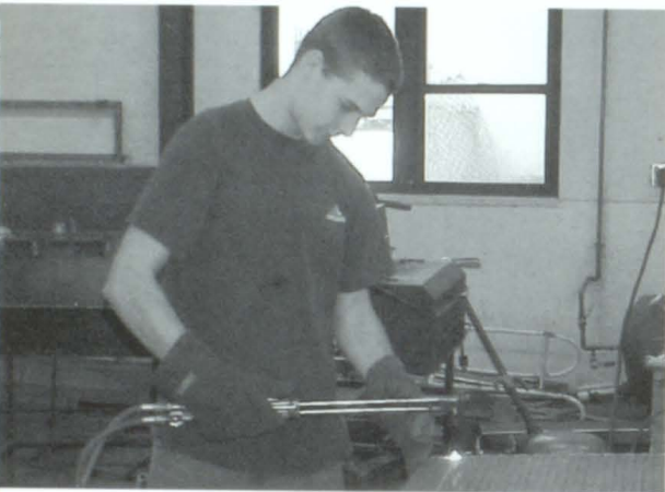
Jay Ruhnke makes a cut on his flat-bed trailer using the cutting torch in ag mechanics. Photo by Crystal Peden
